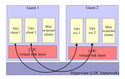
Within a LDom a LDC is instantiated as a single endpoint (unless the LDC loops back to 685 the same LDom). The identity of the owner of the other endpoint is opaque to the LDom this enables LDCs to be re-connected to other endpoints at will. Conventional attestation protocols may be layered on top of the basic LDC mechanism if the identity of the owner of the other end of a LDC is required. Such attestation is beyond the scope for this document.
