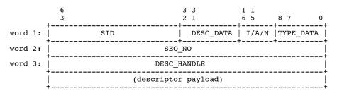
In case of both a DRING\_DATA and DESC\_DATA message, if the receiver gets a data packet out of order (as indicated by a non-consecutive sequence number) then it will NACK the packet and will not process any further data packets from this client. If there are no errors the receiver will ACK the receipt of descriptor ring or descriptor data packets if there is an explicit request by the sender to ACK a data packet by setting the (A)cknowledge bit in the descriptor.
