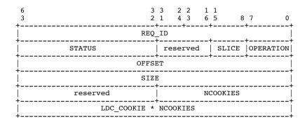
The payload contains the *operation* being performed.
