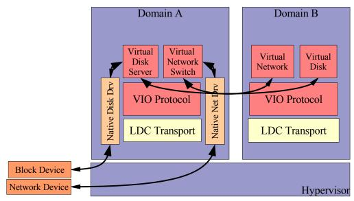
The figure below shows two logical domains with VIO device clients and services communicating with each other using the VIO protocol and layered on top of the underlying LDC framework. Domain A has exclusive access to local physical devices through native device drivers and exports access to these devices over the LDC connection to domain B. VIO data transfer
